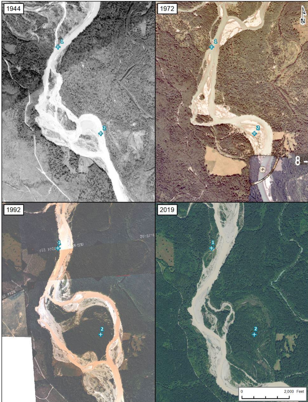
Figure 12. Time series of channel change between 1944-2019 showing abandonment of the channel feature between RM 1 and RM 2.
