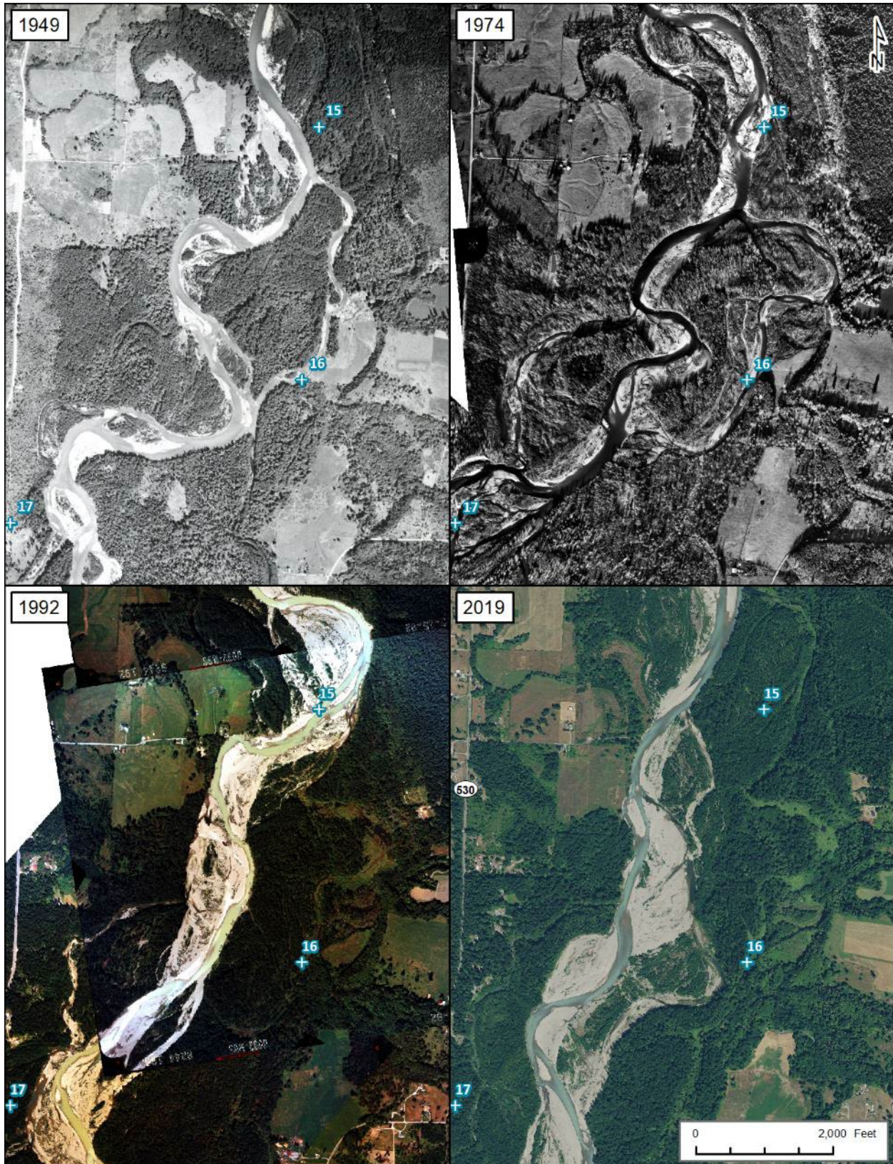
Figure 35. Time series of historical channel changes in reach SA050 between RM 15 and RM 17.
