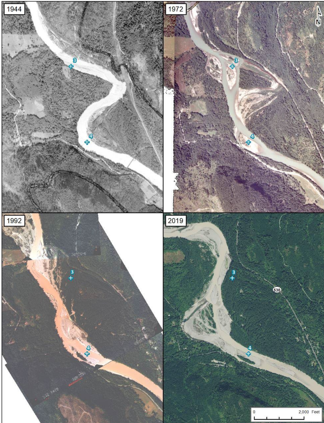
Figure 13. Time series of historical channel change 1944-2019 showing two sequences of bend cutoffs between RM 3 and RM 4.
